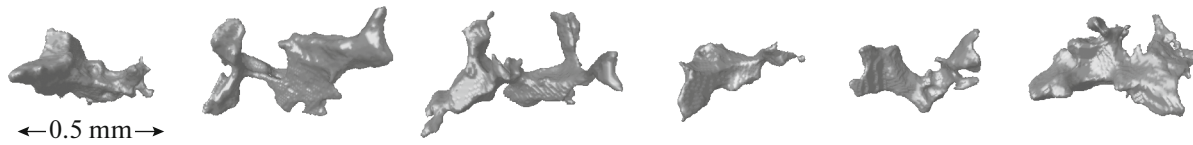
Fig. 13. 3D models of the largest particles of the sulfide phase in the plagioclone samples.
