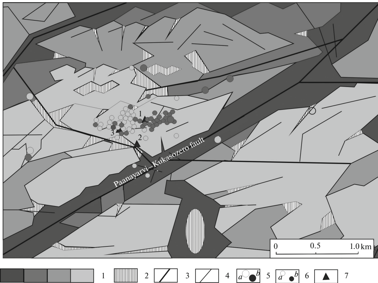
Fig. 7. A map of the block divisibility of the Paanayarvi area and the spatial distribution of ME epicenters recorded in July 4–11, 2004. (1) height gradation of the upper surfaces of morphostructurally visible blocks with differentiation along height at intervals of ~10 m; (2) zones of local tension—separations that can act as asperities during relative block movements; (3) faults that separate the blocks; the faults are expressed as large relief forms; (4) intrablock faults that are expressed as small morpho-sculptural forms; (5) ME epicenters of energy over 100 J: with dominant signal frequency 2–9 Hz ( a ) and 9–40 Hz ( b ); (6) ME epicenters with source energy below 100 J: with dominant signal frequency 2–9 Kz ( a ) and 9–40 Hz ( b ); (7) site of seismic observation and its identification number.
