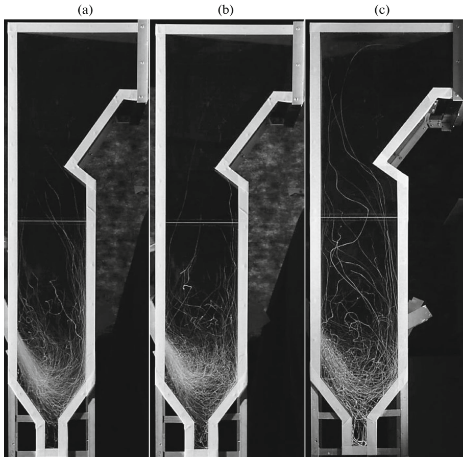
Fig. 3. PCB jet motion trajectories in section I–I: (a)—without restriction orifices; (b) with restriction orifices; and (c) with restriction orifices and closed GOBs.
