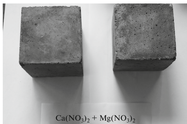
Fig. 4. State of cement concrete specimens prior to test.
