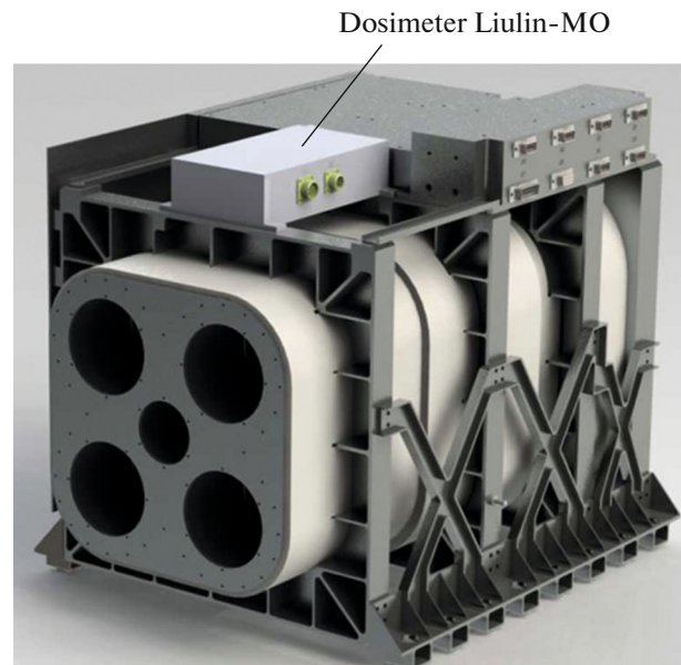
Fig. 2. Location of the Liulin-MO dosimeter on the FRENDD device.
