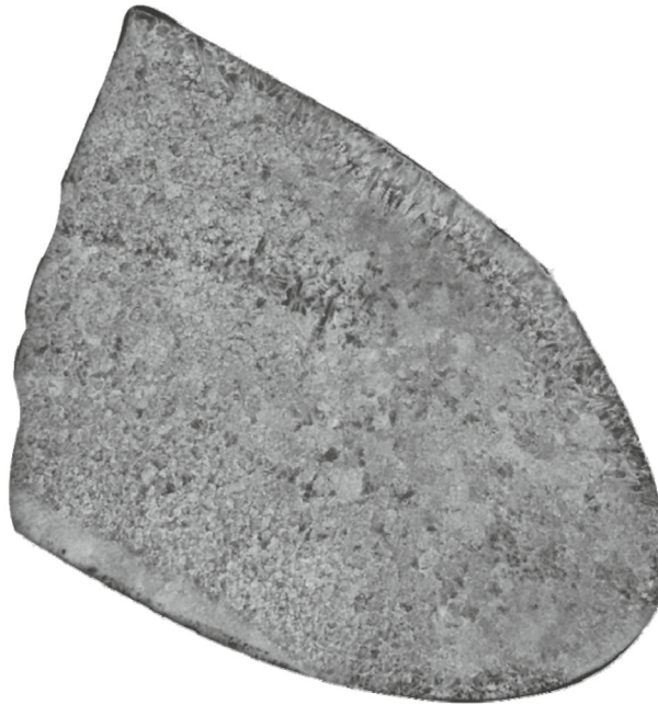
Fig. 4. Cross section of the welded joint formed at a current of 30 A.
