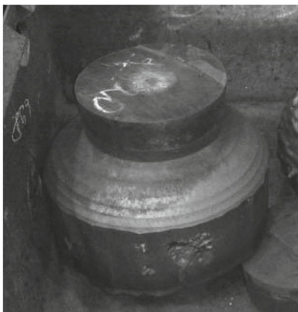
Fig. 3. Retained incompletely melted part after VAR of a consumable electrode made of 03Kh18K8N5T steel 380 mm in diameter in a DSV-6.3 furnace.
