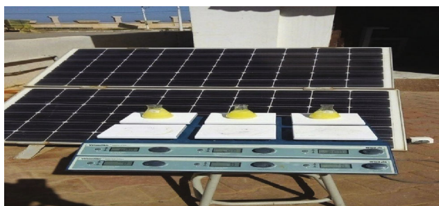
Fig. 2. Schematic representation of the experimental setup used for tartrazine; degradation assays under sunlight radiation.
