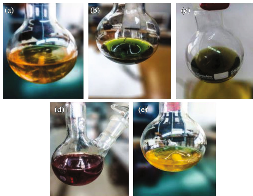
Fig. 1. Aspect of the gel of TiO 2 doped materials: (a) Pure TiO 2 , (b) Cr–TiO 2 , (c) Co–TiO 2 , (d) Fe–TiO 2 , and (e) Zr–TiO 2 .
