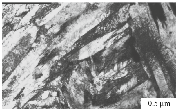
Fig. 2. Structure of carbide-free bainite in 14Kh2H2GMF steel after cooling from 870°C at a rate of 5°C/min.
