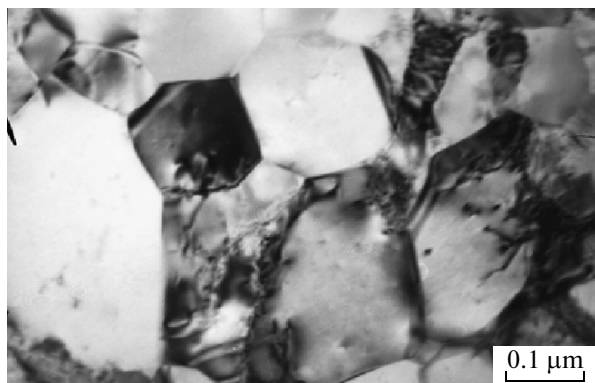
Fig. 4. Microstructure of commercial-purity copper at the stage of the complete dynamic recrystallization (10 rev, \ln Z = 37.2 , e = 8.1 , \omega = 1 rpm).
