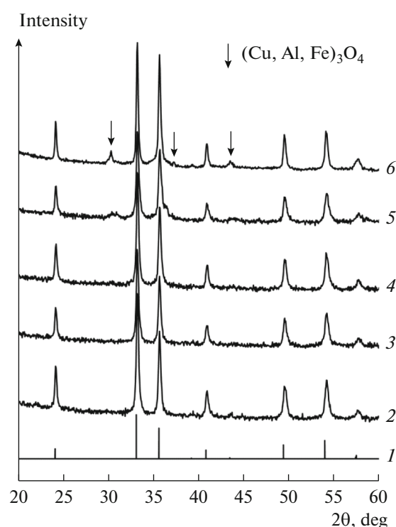
Fig. 3. Diffraction patterns of the Cu–Fe–Al nanocomposite catalysts containing different amounts of copper: (1) \alpha\text{-Fe}_2\text{O}_3 (PDF 330664), (2) \text{Fe}_{82}\text{Al}_{18} , (3) \text{Cu}_3\text{Fe}_{79}\text{Al}_{18} , (4) \text{Cu}_5\text{Fe}_{78}\text{Al}_{17} , (5) \text{Cu}_8\text{Fe}_{75}\text{Al}_{17} , and (6) \text{Cu}_{10}\text{Fe}_{74}\text{Al}_{16} .
