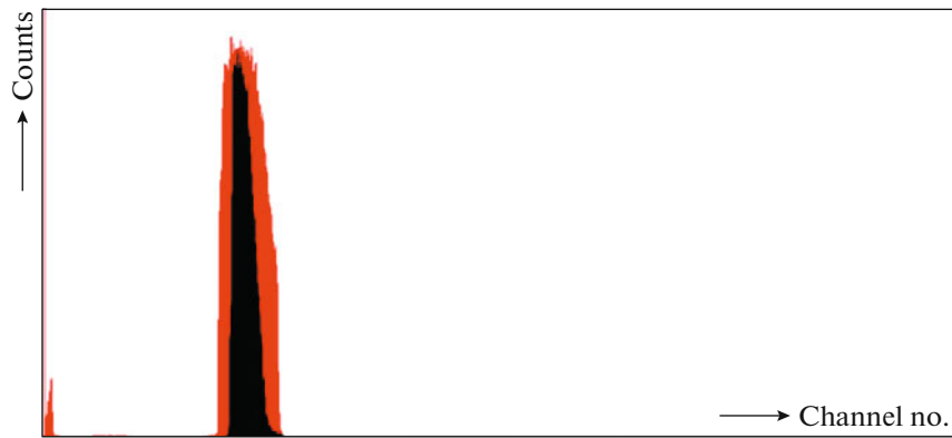
Fig. 10. Comparison of the spectra: gated photopeak (red), timing processed photopeak (black).
