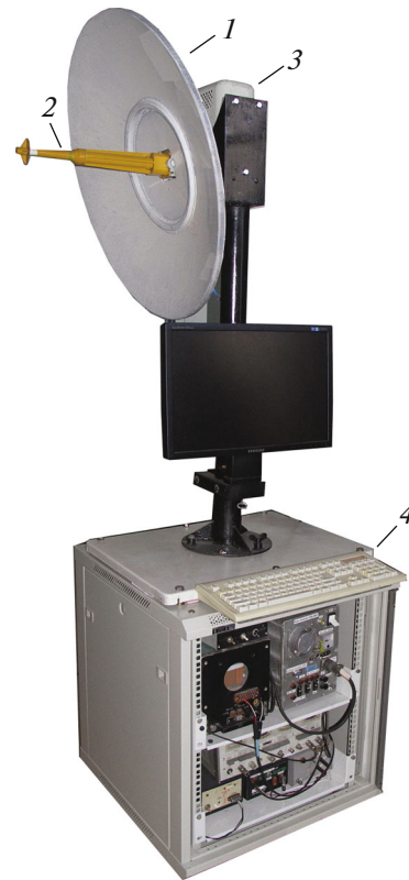
Fig. 6. The appearance of the prototype of the onboard aircraft equipment based on the Groza 26 aircraft radar station: (1) mirror antenna; (2) exciter with a built-in ferrite rotator of the polarization plane; (3) antenna column; and (4) receiving and measuring equipment.
