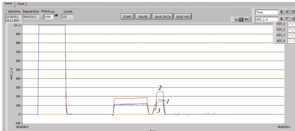
Fig. 6. The current of the ^{32}\text{S} ion beam with an energy of 51 MeV/nucleon, which was measured using the three-lamel probe mounted on the final orbit of the MTs-400 cyclotron. The indications of the ADC_1 – ADC_3 currents correspond to the measurements of the currents from (1) the upper (ADC_1), (2) central (ADC_2) and (3) lower (ADC_3) lamels.
