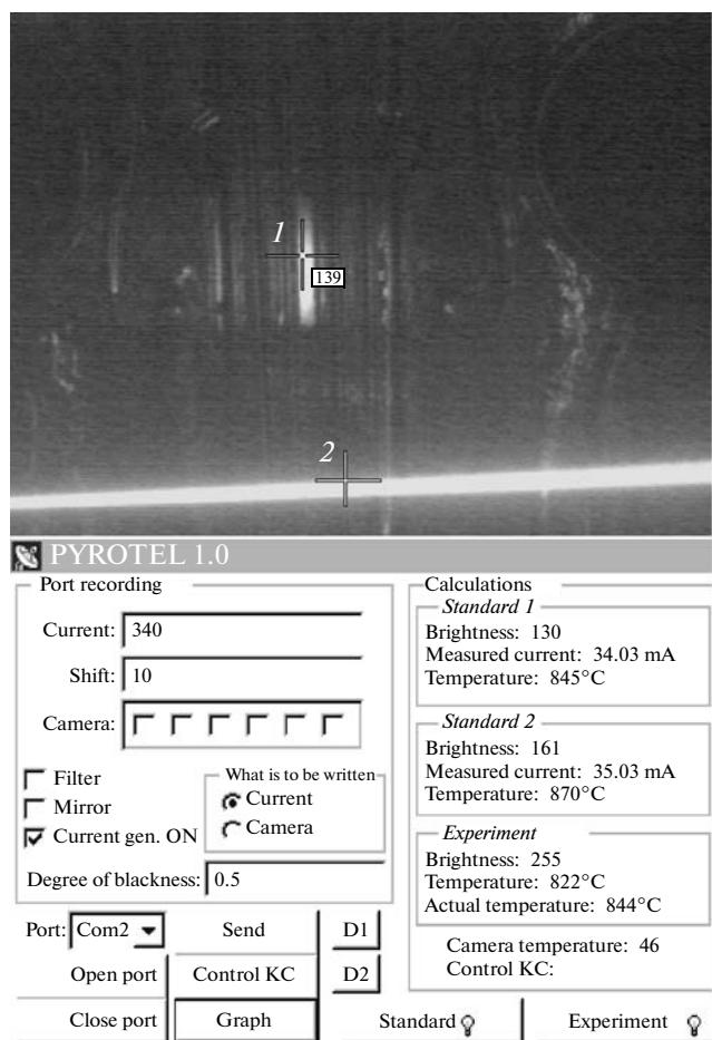
Experimental measurement of the incandescent tungsten strip temperature via a water streak using the TPS (flat streak thickness, 100 mm;  $T_{\text{strip}} = 1000^\circ\text{C}$ ;  $T_{\text{amb}} = 25^\circ\text{C}$ ; and illuminance,  $E = 40 \text{ lx}$ ): (1) tungsten strip of the lamp and (2) filament of the reference source of the brightness temperature.
