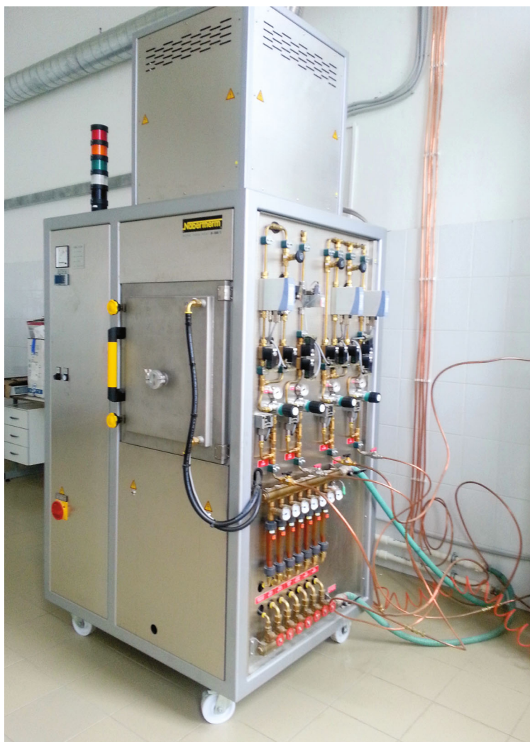
Fig. 1. Photo of a Nabertherm furnace with special additional inlets for CO, SiH 4 , H 2 , and Ar gases.
