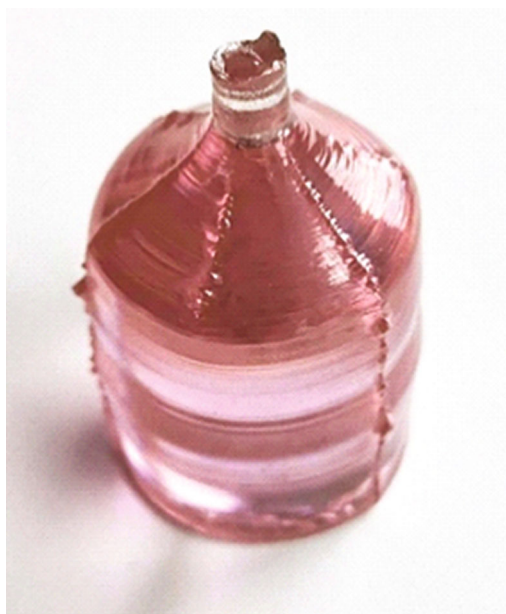
Fig. 2. Appearance of a \text{LiNbO}_3\text{:Zn(2.48 wt \%):Er(0.98 wt \%)} crystal.
