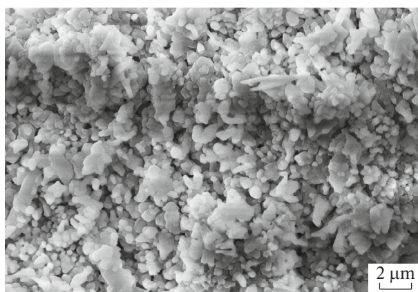
Fig. 6. Microstructure of \text{Si}_3\text{N}_4 prepared using a starting mixture containing 23 wt % Si and 1 wt % \text{Na}_2\text{SiF}_6 .
