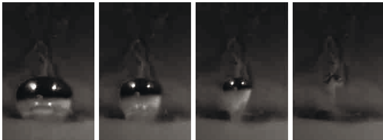
Fig. 9. Collapse of a vapor bubble (lateral view) [124]. Time interval between frames, 100\ \mu\text{s} ; heat-flux density, 1.5\ \text{MW}/\text{m}^2 ; underheating value, 76^\circ\text{C} . The water is still, and the surface is an aluminum plate with \text{Al}_2\text{O}_3 coating.
