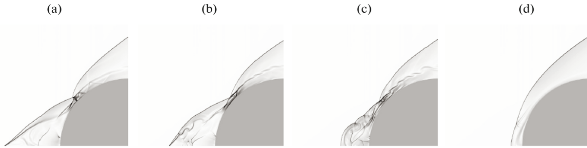
Fig. 4. Schlieren patterns of flow at different time instances [49]: (a) \tau = 2.88 \times 10^{-4} s, (b) 7.54 \times 10^{-4} s, (c) 8.68 \times 10^{-4} s, and (d) 1.1 \times 10^{-3} s.
