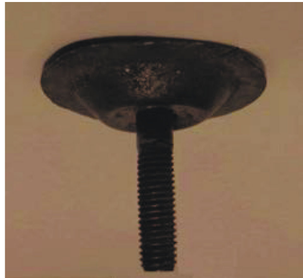
Fig. 2. Gas burner cover for domestic stoves with the heat-transfer enhancer in the form of the thread.
