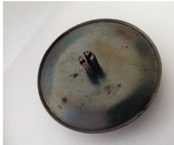
Fig. 4. Gas burner cover for domestic stoves with the heat-transfer enhancer in form of the rod with a filament and widening slot-type gaps.
