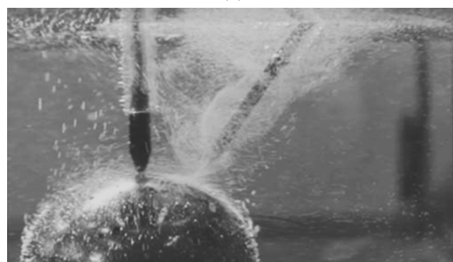
Fig. 8. Vortex formation in a solution of acetic acid in the orientation of the positive movable electrode at 54^\circ to the horizontal plane; (a) pattern of vortex formation: (1) magnet holder, (2) movable electrode, (3) permanent magnet, (4, 5) Lorentz force \mathbf{F}_L acting on the ions of the electrolyte, and (6) vortex motion trajectory; \mathbf{B}_m , magnetic induction field produced by a magnetic sphere; \mathbf{B} , induction of the magnetic field generated by a current-carrying conductor; \mathbf{V} , velocity vector of acetate ions under the Coulomb forces; (b) visualization of vortex formation.
