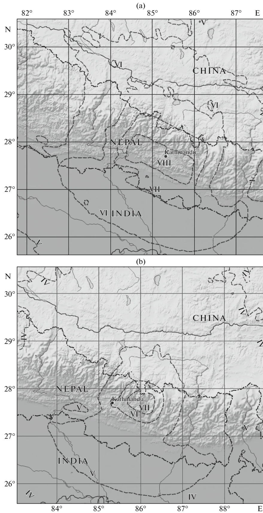
Fig. 3. Isoseismal map for highest shaking of mainshock (a) and strongest aftershock of May 12, 2015 (b) based on USGS data [30].
