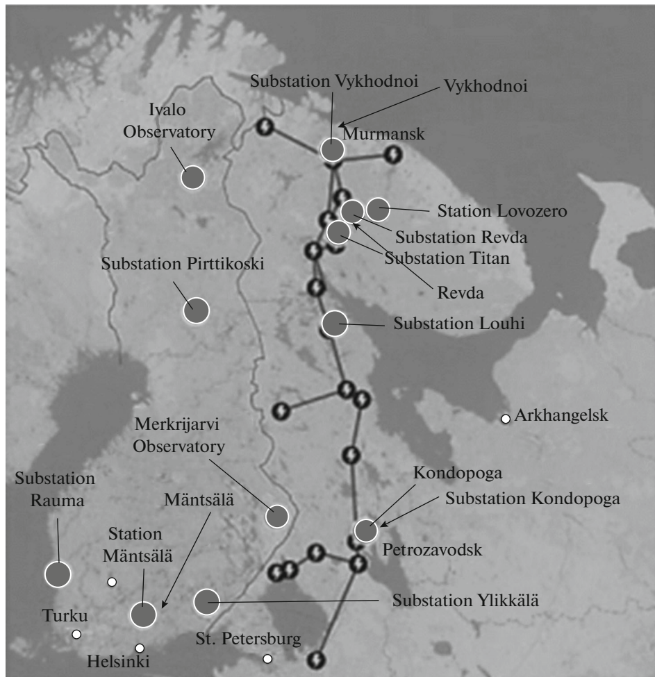
Fig. 1. A schematic of measuring instruments in the EURISGIC project: the circles denote the nearby observatories measuring the geomagnetic field and the GIC recording substations. The arrows and labels indicate the substations used in this study.
