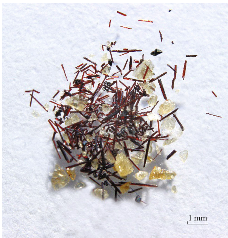
Fig. 3. Own Ln phases in the hematite crystallization field (run 4). Lamellar crystals are hydrous oxychloride of mainly light and medium Ln , acicular crystals are oxyhydroxide of Fe and medium–heavy Ln , and equant rhombic crystals are hematite.
