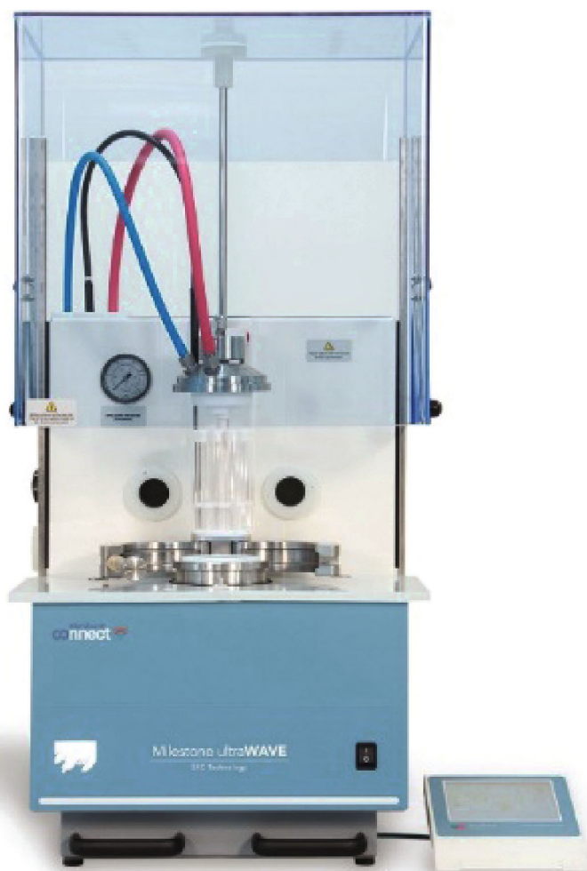
Fig. 1. UltraWAVE microwave system (Milestone, Italy).
