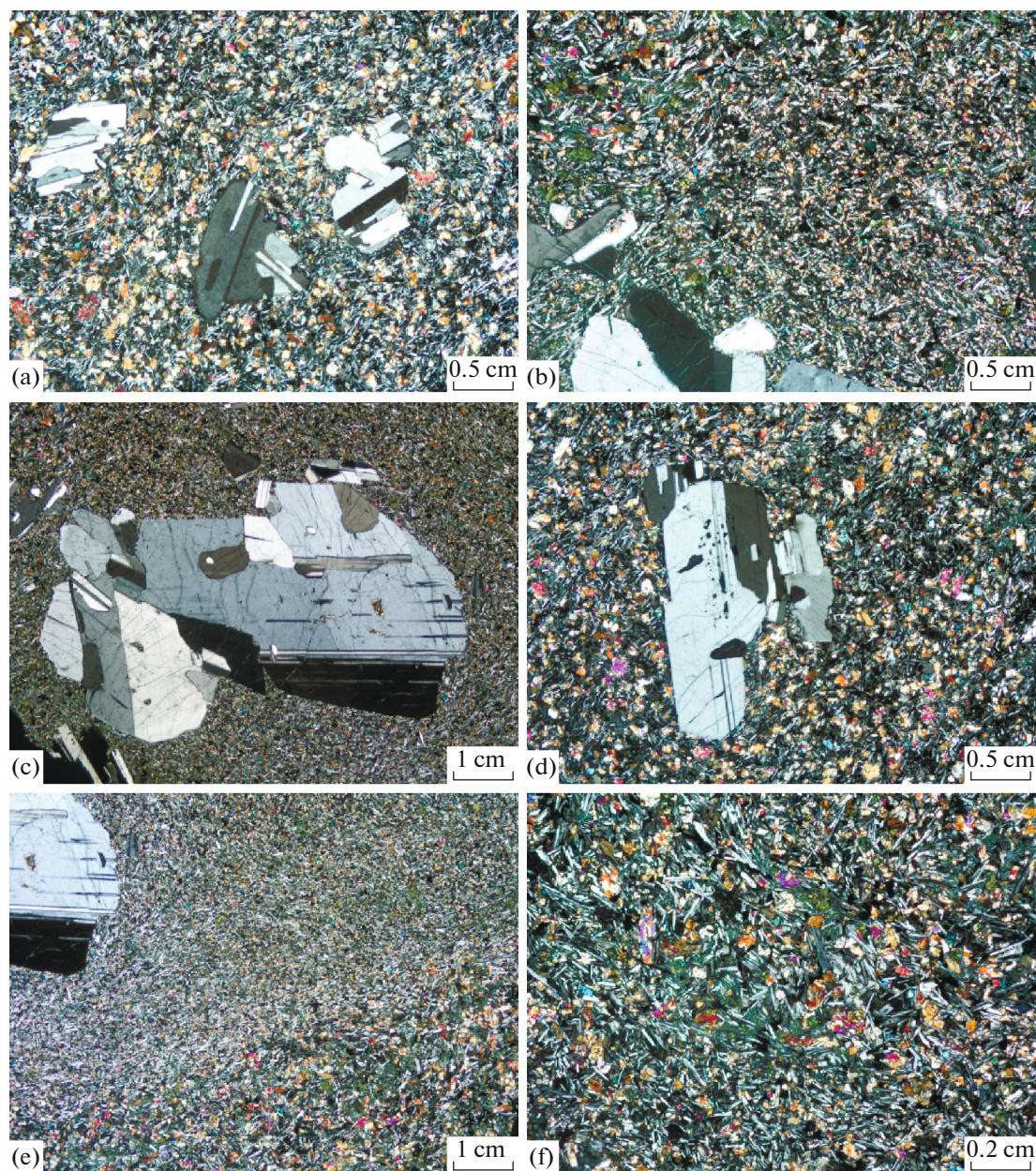
Fig. 3. Micrographs of basalts from the Nadayansky Flow: (a, b) porphyritic textures of the rocks; (c, d) glomerophyric plagioclase aggregates; (e, f) plane-parallel groundmass structure.
