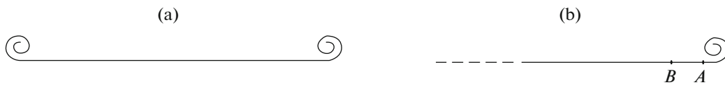
Fig. 6. Evolution of the vortex wake behind an elliptically loaded wing; (a) plane section, (b) the vicinity of the right vortex, on its scale the left vortex is located at infinite distance from the right vortex.
