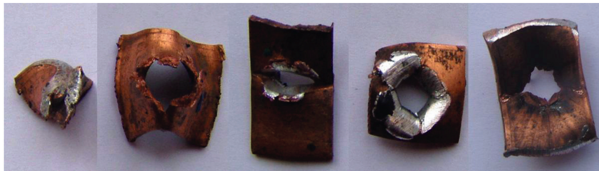
Fig. 6. Visual appearance of the witness plates after exposing the target to laser radiation that initiates the aluminized explosive.
