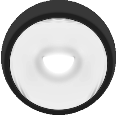
Fig. 5. Stabilization of the combustion wave: the igniting region S is a semicircle ( |r| < 160 and \pi < \varphi < 0 ): \theta_{\text{ign}} = 1 , \tau_{\text{ign}} = 4500 ; R_0 = 600 , \theta_0 = -9 , \text{Ar} = 0.08 , \text{Ph} = 0.4 , \theta_l = -0.5 , and \tau = 4157 .
