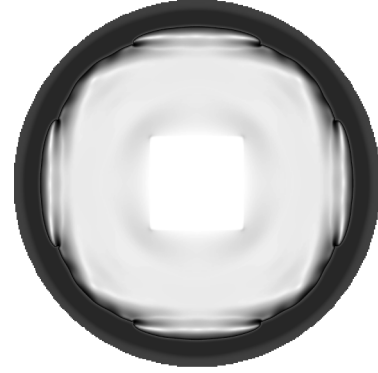
Fig. 6. Effect of the phase transition on the multi-hot-spot combustion mode (the igniting region S is a 150 \times 150 square): \theta_{\text{ign}} = 1 , \tau_{\text{ign}} = 5000 ; R_0 = 600 , \theta_0 = -9 , \text{Ar} = 0.08 , \text{Ph} = 0.3 , \theta_l = -1.5 , and \tau = 5100 .
