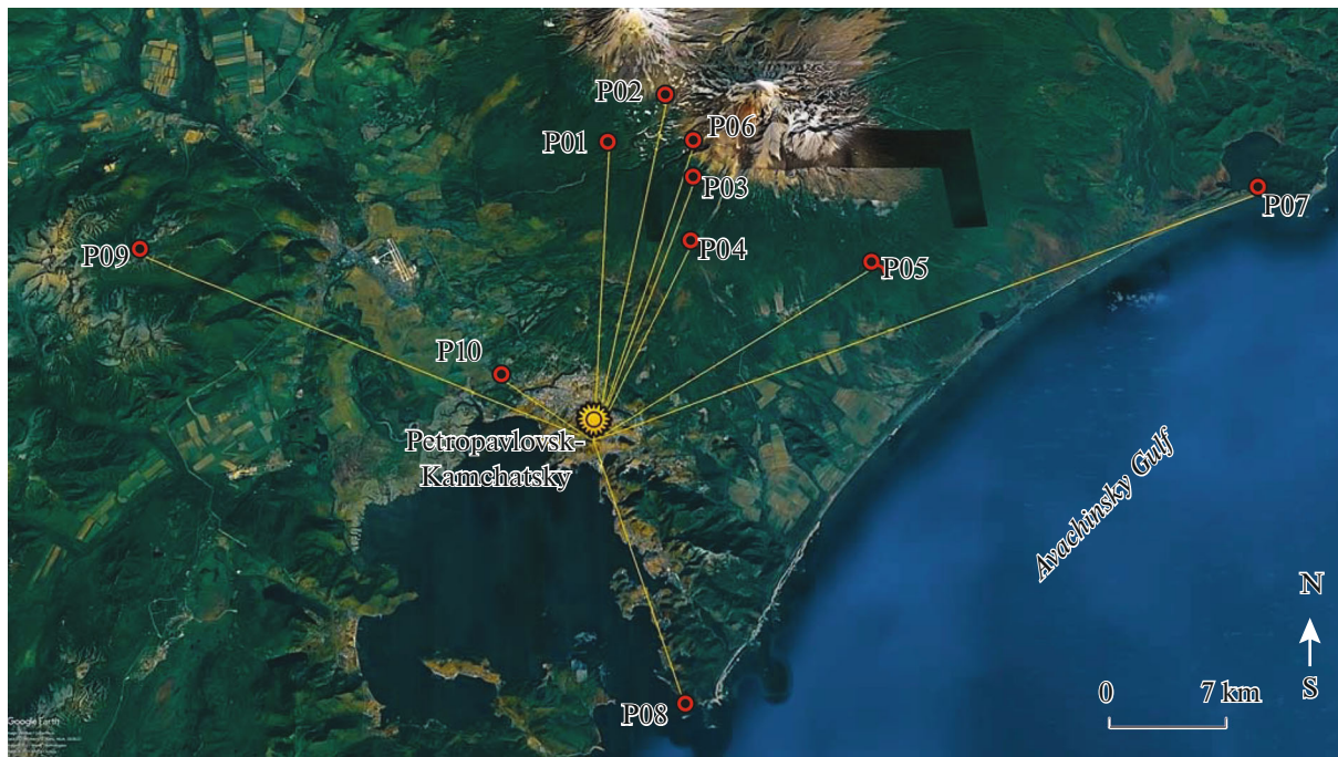
Fig. 3. A schematic of the arrangement of optical distance lines for measurements at the Mishennaya observatory (Petropavlovsk-Kamchatsky). P01–P10 are the stations with corner reflectors.
