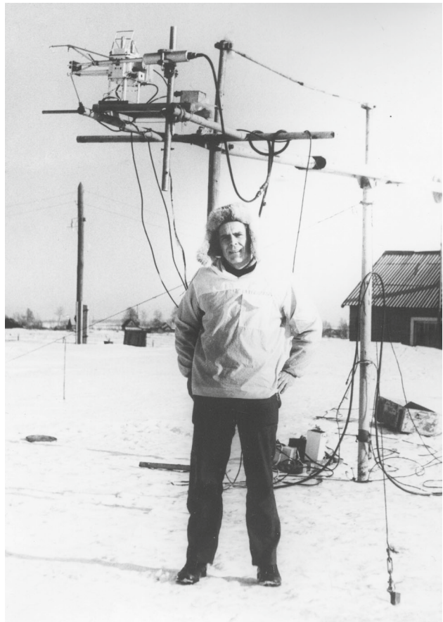
Fig. 13. Measuring system in operating position during the winter expedition in Koltushi (anemometer, hygrometer, and resistance thermometer).
