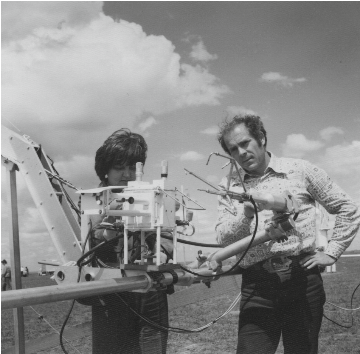
Fig. 15. L.G. Elagina and B.M. Koprov are mounting an acoustic anemometer and a hygrometer during the International Turbulence Comparison Experiment in Australia.
