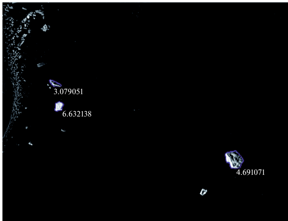
Fig. 11. Height of icebergs and their fragments calculated by shadow length on the sea surface. The EROS-B image as of September 3, 2012; digits show height values. ImageSat Int., SCANEX.
