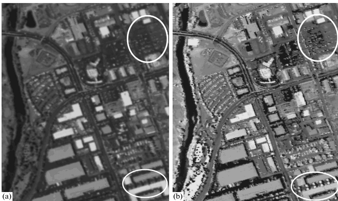
Fig. 6. Results of aviation hyperspectral image processing: (a) averaging of all HSI spectral channels, (b) integration.
