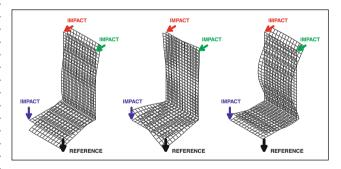
Now we can see that the single reference point is sufficient to adequately observe all the modes of interest—and only one direction is necessary to accomplish this. Of course, if more references are used this is totally acceptable and is definitely a better way to test the structure—but these extra references are not necessarily needed in order to extract modes shapes that are three dimensional in nature.
