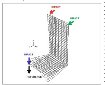
And if the third mode is considered with the reference accelerometer located at the lower corner in the *z*-direction, all three impact locations on the structure have significant response at this point for this mode.
