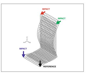
Now the real question is if there is ONE reference location that can be selected that will adequately capture the dynamic characteristics of the structure for all the modes of interest. For this case, it seems reasonable that the lower corner of the structure in the *z*-direction is sufficient to observe all of the modes for this case.
