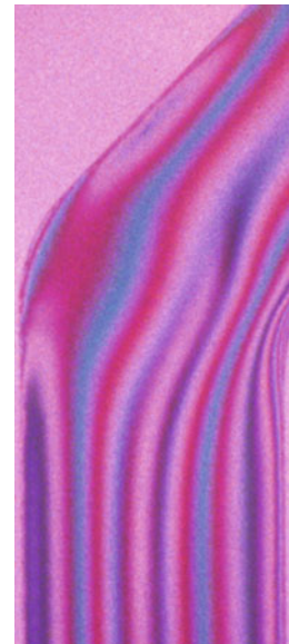
Detail from light-field photoelastic interferometry fringe pattern obtained using simultaneous illumination from two laser sources: Argon at 488 nm (turquoise) and Helium-Neon at 633 nm (red). The granular appearance is caused by laser speckle. Photo by Gary Cloud, March 2003.
