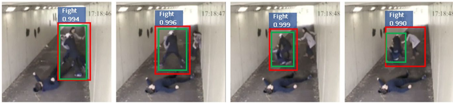
Fig. 3 An example of action (fighting) detection results for T-CNN. The green boxes indicate the ground truth and the red boxes indicate the predicted bounding boxes for action “fighting” generated by CV. The numbers denote the probabilities associated with a correct label being assigned to the action
