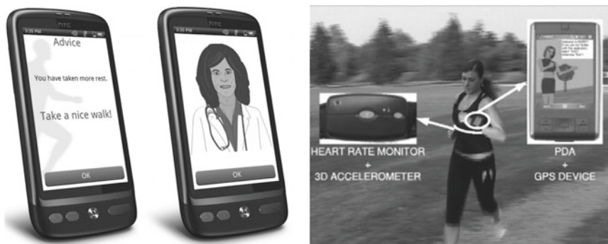
Fig. 17.2 Text-based and ET interfaces to promote walking (left) (Klaassen et al. 2013) and the MOPET system for outdoor fitness (right) (Buttussi et al. 2006; Buttussi and Chittaro 2008)
