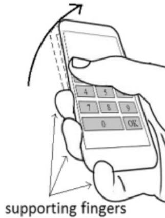
Fig. 26.5 Supporting fingers push the phone upwards to touch a digit Source: Author's own design
