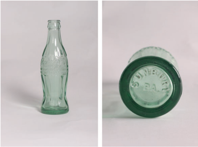
Fig. 4.17 (a, b) This six-oz green Coca-Cola bottle (left) was manufactured in Sunbury, PA (right), under the Dec. 25, 1923, registered patent. In a competitive soda industry full of generic, straight-sided bottles, the curved bottles stood out, and helped establish the Coca-Cola brand worldwide
