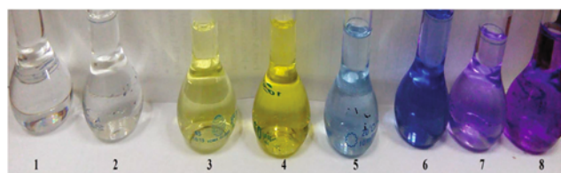
Fig. 15 Colour response of SP/MC from the solvent stimuli: 1 – toluene, 2 – 1,4-dioxane, 3 – acetonitrile, 4 – acetone, 5 – DMF, 6 – DMSO, 7 – EtOH, and 8 – methanol.
