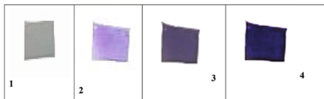
Fig. 14 SP embedded in PMMA film (1) – before immersion in EtOH, and after immersion in EtOH for (2) – 30 min, (3) – 1 h and (4) – 2 h.
