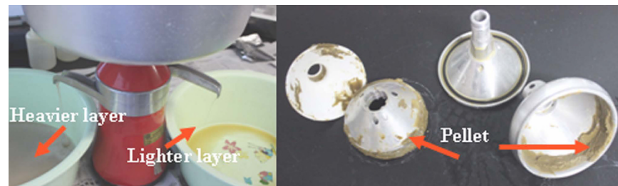
Figure 2. Three phase electrical cream separator (lighter, heavier and pellet).
