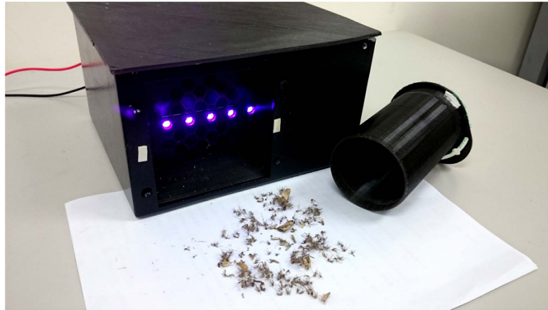
Figure 6. The UV LED bug zapper constructed for experiments of the study.
