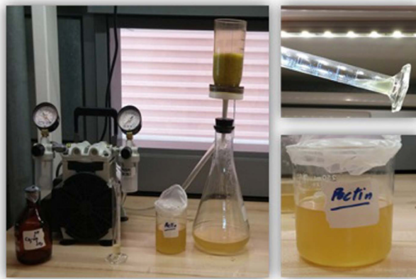
Figure 2. Experimental set-up used for single step green and facile extraction of pectin (left); a qualitative test shows presence of active pectin as white gelatinous shining phase in the bottom of tilted beaker (right).
