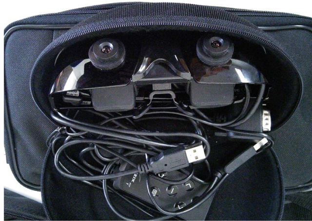
Figure 21. The HMD utilised for this work, with video see-through capabilities.
