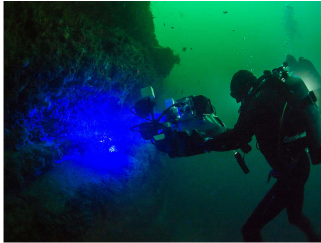
Figure 7. Scientific biofluorescent imaging camera and lighting system developed to obtain 4 K imagery shown underwater in Scripps Canyon, San Diego, CA. Image courtesy of Kyle McBurnie.
