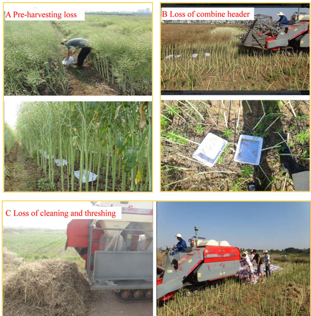
Figure 5. Schematic operation for determination yield losses in the study. (A) loss of naturally pod shattering pre-harvesting; (B) loss of combine header; (C) loss of cleaning and threshing.
