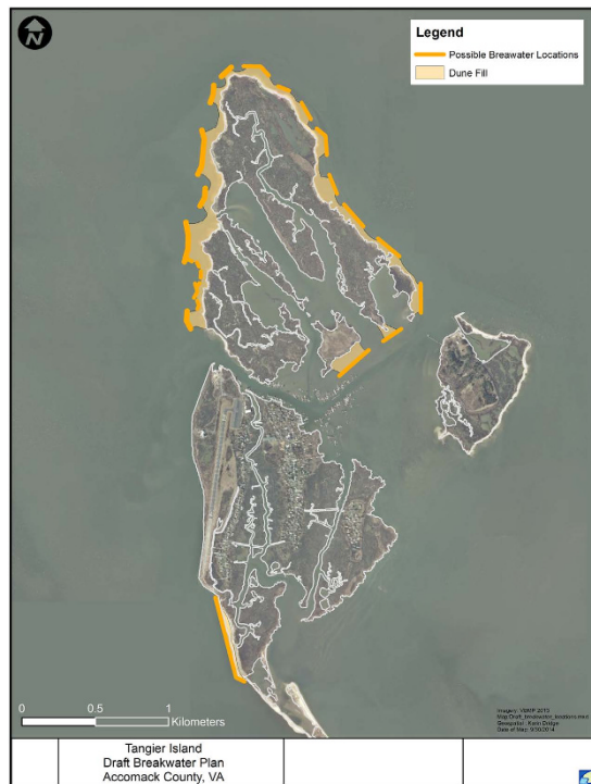
Figure 5. Conceptual protection/restoration plan to maintain the remaining landmass of Uppards and Tangier Island. Map created using ESRI ArcGIS, ArcMap 10.1. Source: Esri, DigitalGlobe, GeoEye, Earthstar Geographics, CNES/Airbus DS, USDA, AEX, Getmapping, Aerogrid, IGN, IGP, swisstopo, and the GIS User Community. For more information on this map, including the terms of use, visit: http://goto.arcgisonline.com/maps/World_Imagery .
