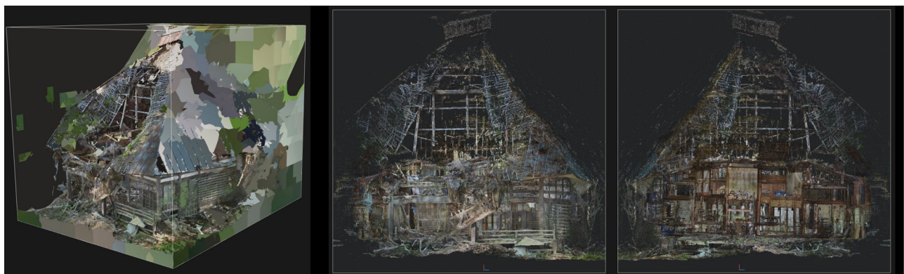
Fig. 6 | Views of a Photogrammetry model of Anyoji temple constructed using RealityCapture showing the skin and structure of the building, including internal spaces filled with furnishings.
