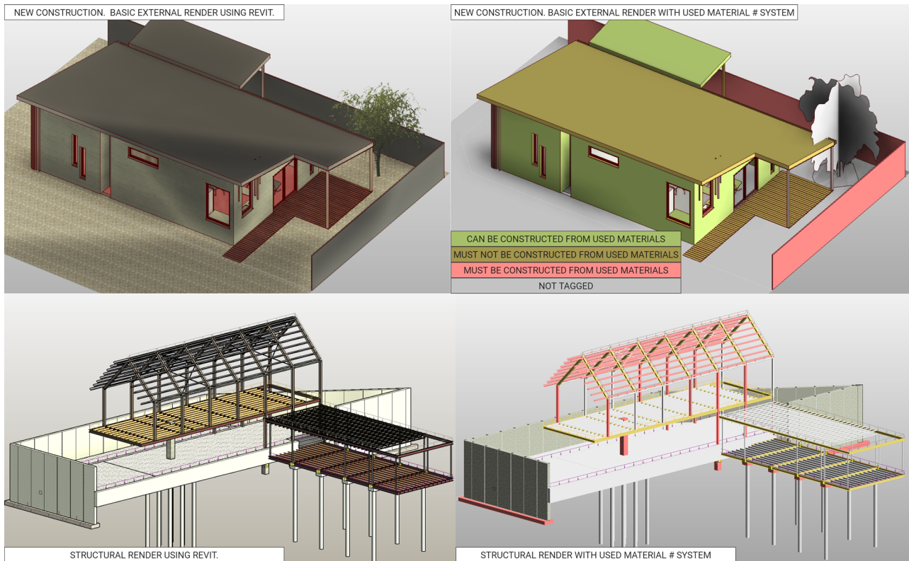
Fig. 2 | Visualisations of a building design using the exterior of a residential building and the Revit template construction file for an interior structure of a commercial building. The BIM hashtag filter is applied to highlight the intent to
