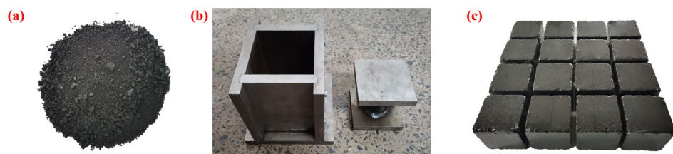
Fig. 2. Sample mold and soft coal samples: (a) raw coal; (b) sample mold; (c) part of coal samples.
